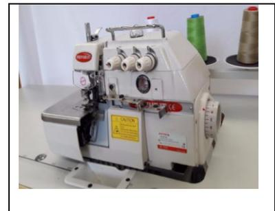
**Figura 27: Máquina overlock**
